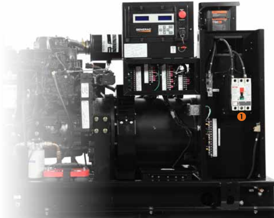
The CCI on a 50kW diesel-fueled generator for the telecom industry. Key to making installation as easy as possible was the repositioning of the circuit breakers (1) to provide more room for cable regrouping, and to allow the cables to run straight into the breaker bays.
